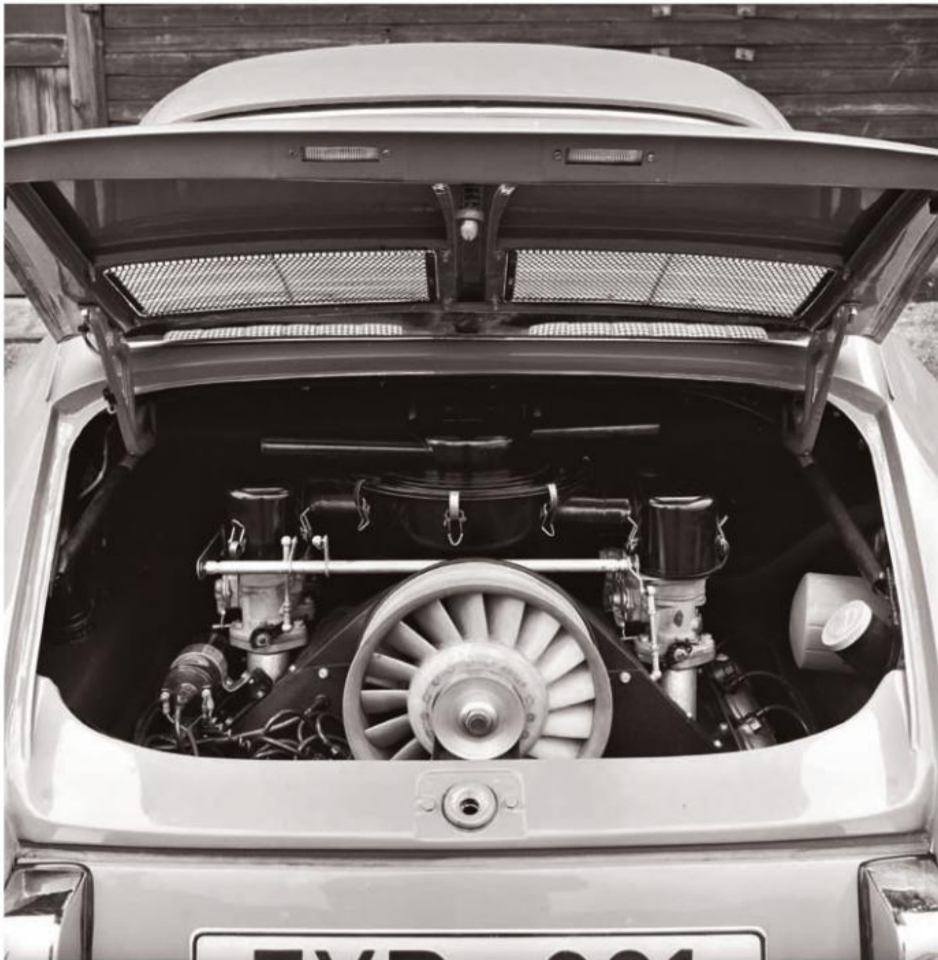
The Typ 901 engine displaced 1,991cc, based on bore and stroke of 80mm and 60mm. The flat six-cylinder configuration developed 130 brake horsepower with fuel fed through two triple-throat Solex overflow carburetors.
