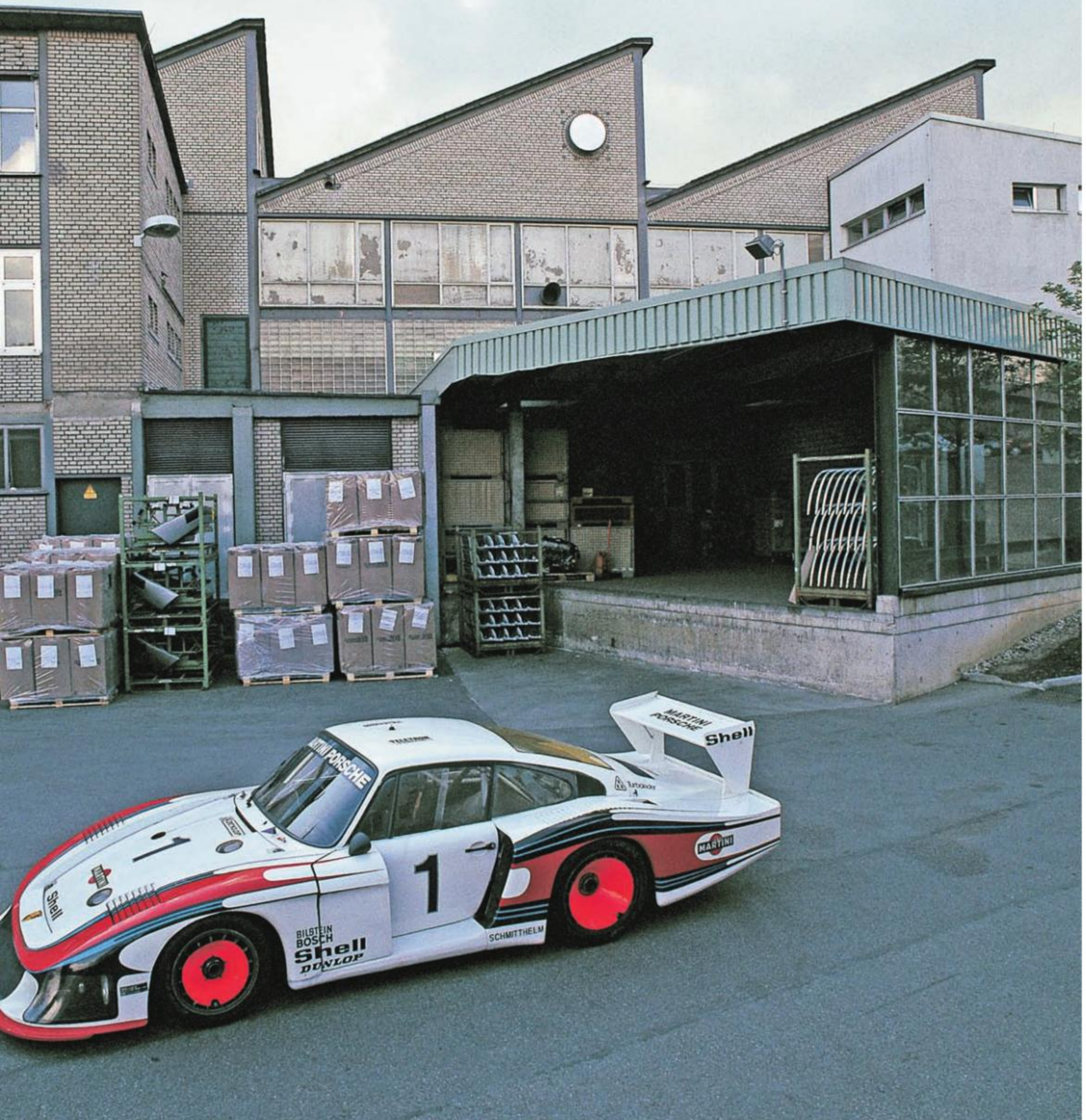
At Le Mans, along the Mulsanne Straight, Rolf Stommelen touched 227.5 miles per hour (366 kilometers per hour) in practice with full boost delivering 900 horsepower. For the race, drivers dialed it back to 750 horsepower, and drivers Bob Wallek, Jürgen Barth, and Jacky Ickx brought the car home in second overall.
