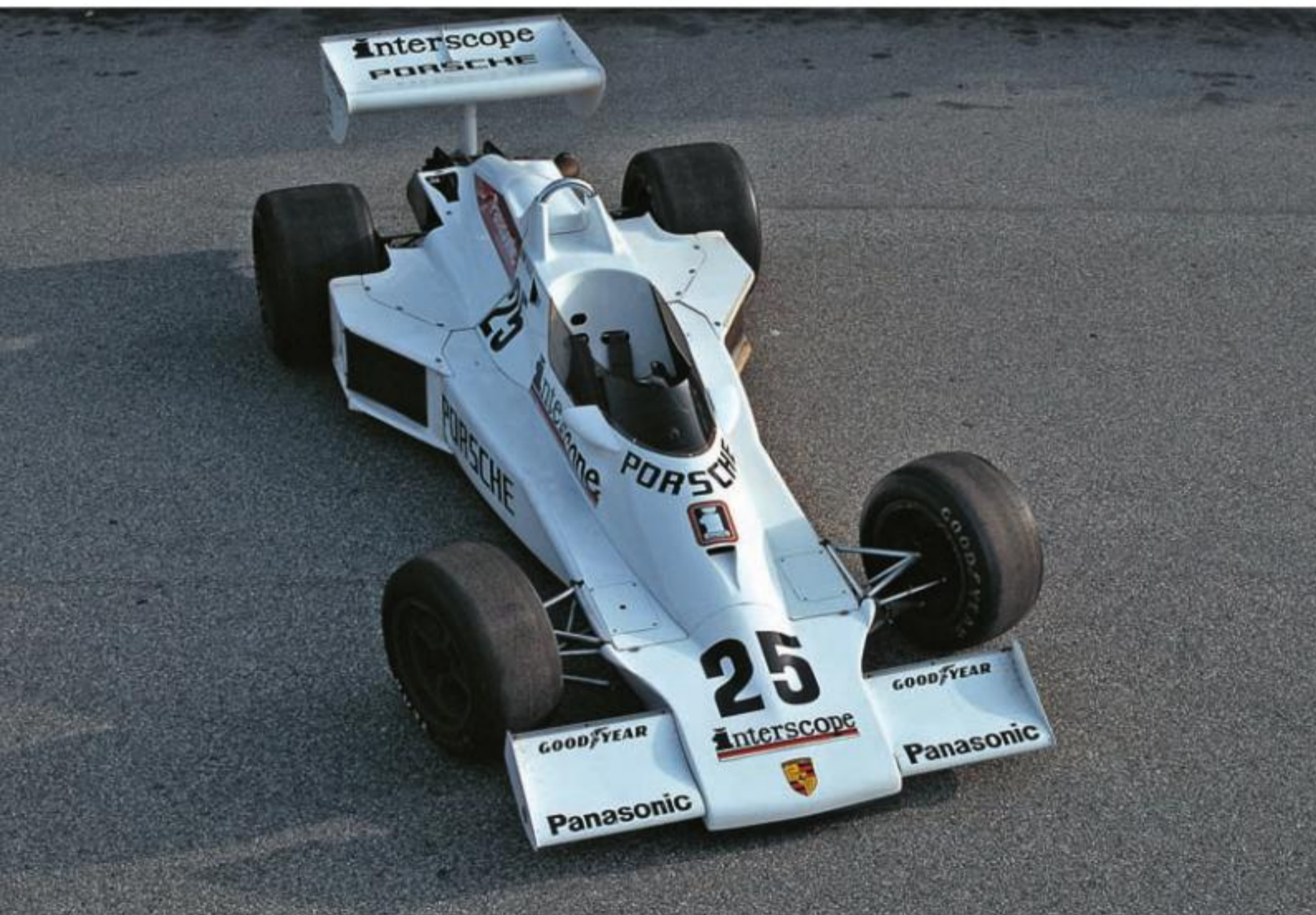
The state of the art in 1980 meant fairly clean and simple bodies. A front and rear wing were about as sophisticated as air management got in those days at Indianapolis.
