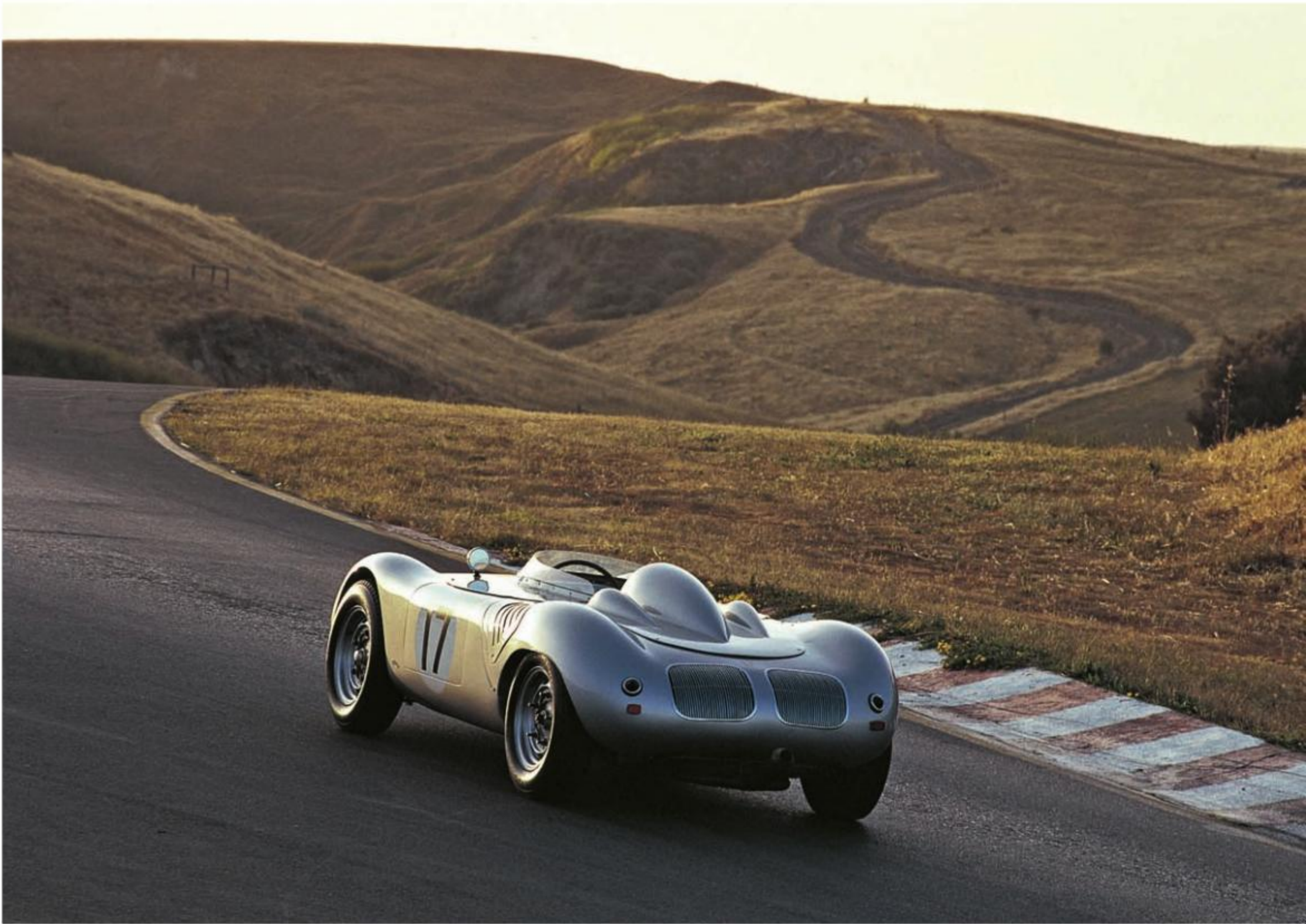
Wendler produced the sleek aluminum bodies for the RSKs. Conversion from left side to center steering took about four hours.
