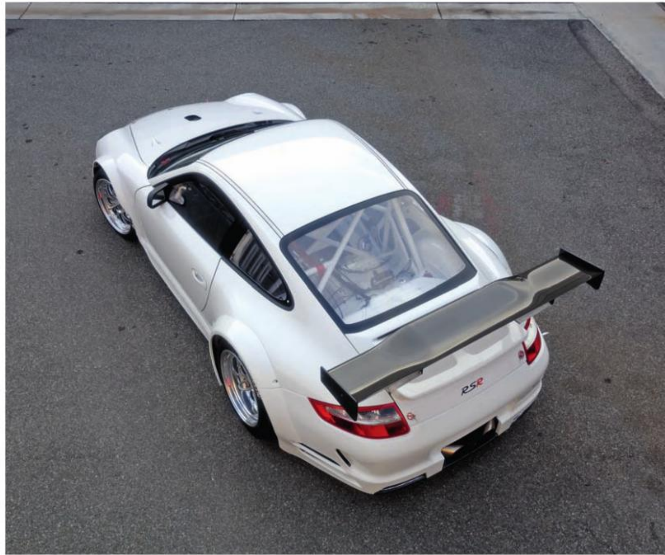
Intense attention to airflow over the car and into and out of radiators, brakes, and engine improved aerodynamic efficiency by 7 percent over the 996 version. Porsche assembled 35 of the cars for the 2007 season.
