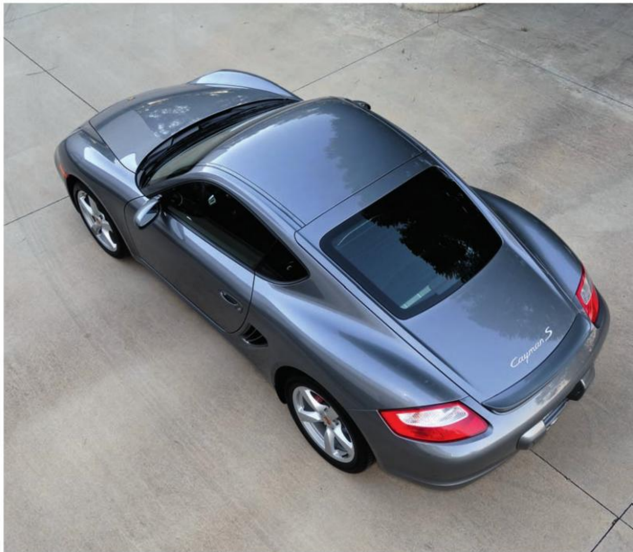
The subtle rear lip past the end of the hatchback is an aerodynamic wing that rises from the body at speeds above 75 miles per hour (120 kilometers per hour). Drivers also can manually control it from inside the car.
