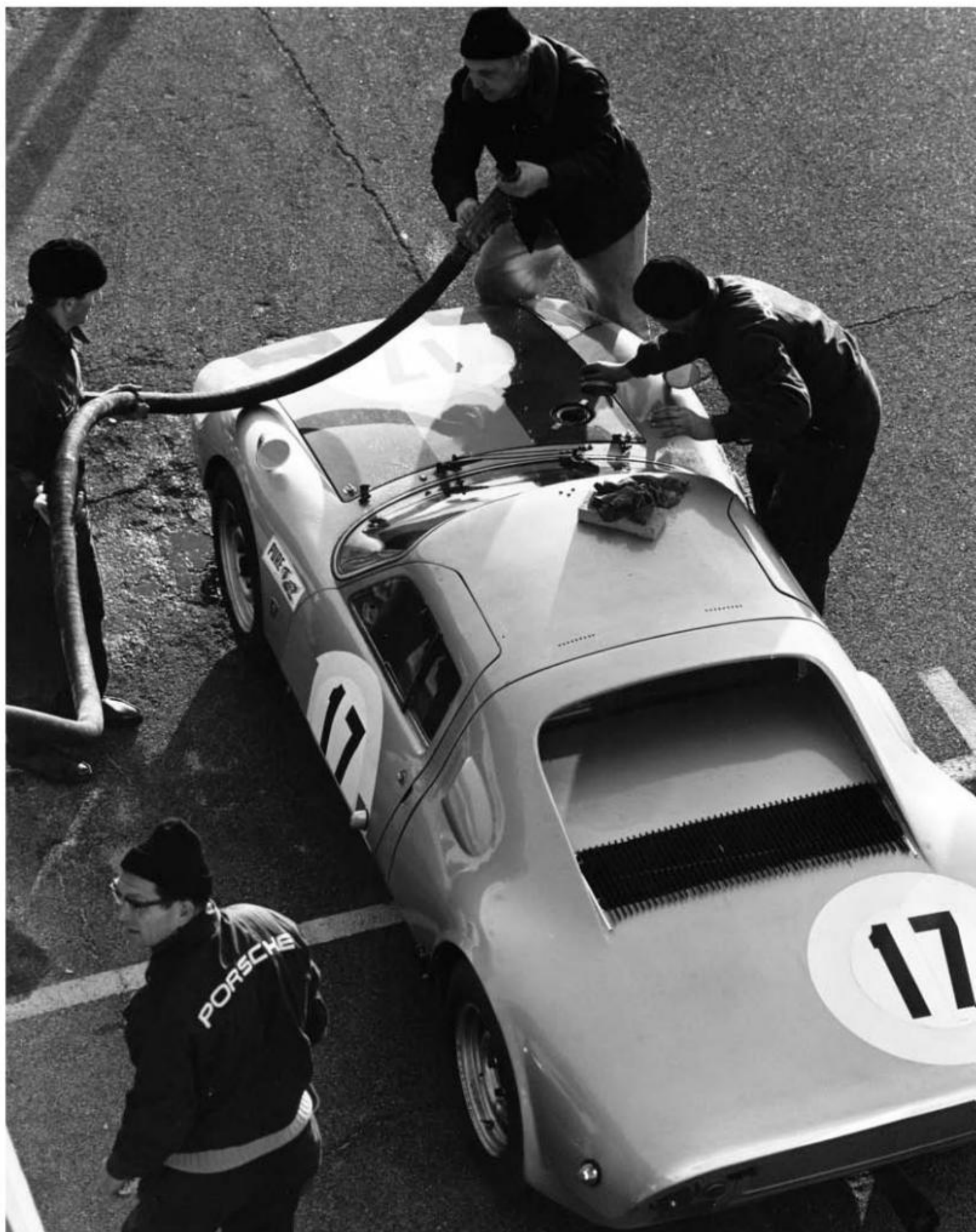
From every angle the 1964 Typ 904 Carrera GTS was visually striking. That it also won race after race from its debut onward was testimony to Gerhard Schröder's ladder-frame chassis, Hans Tomala's concept to sheath the car in fiberglass, and the latest versions of Ernst Fuhrmann's Carrera flat-four engine.
