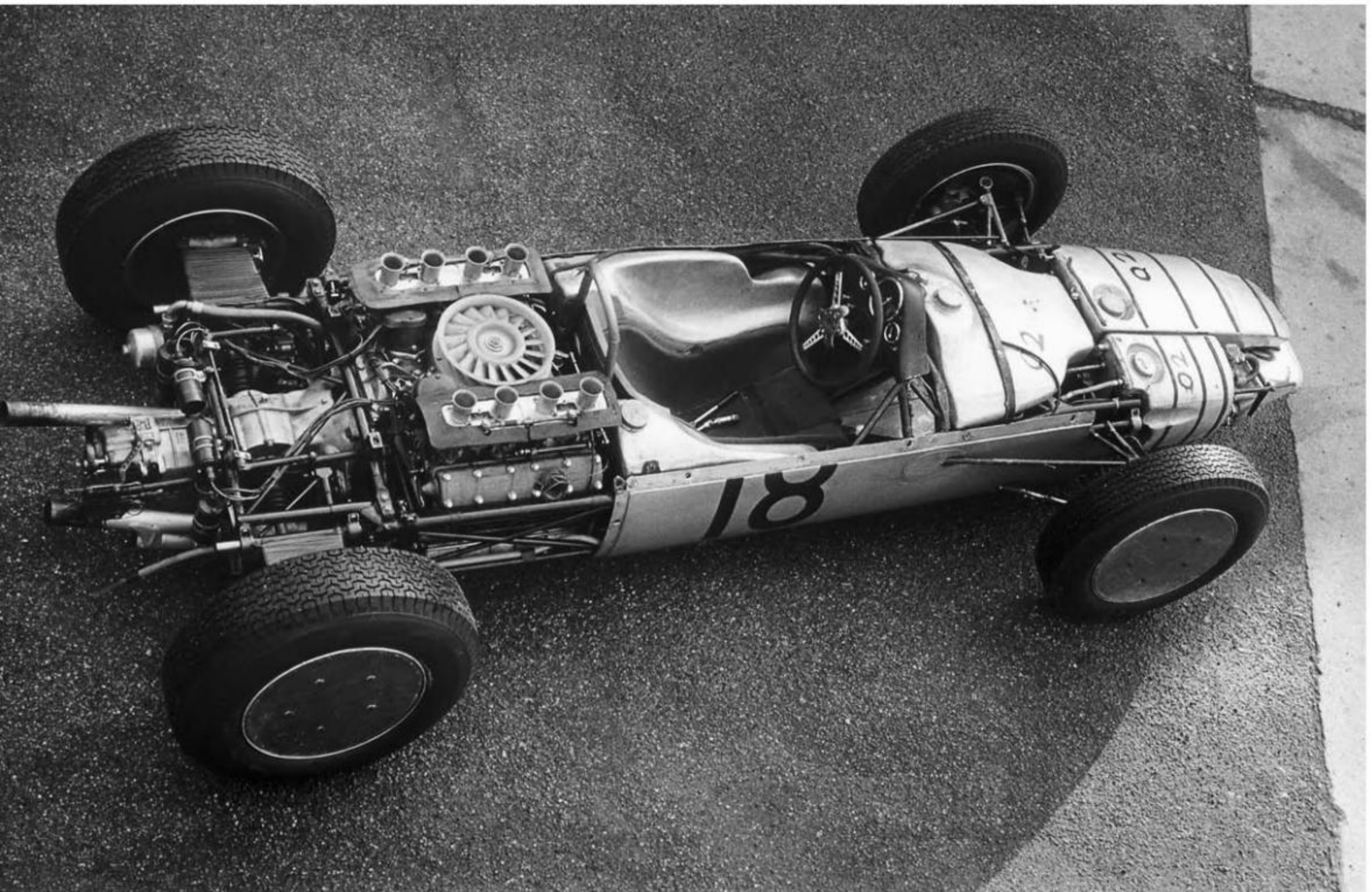
Typical of the time, drivers Dan Gurney and Jo Bonnier sat cradled between fuel tanks on the 1,001-pound (455-kilogram) car. The complicated 1.5-liter Typ 753 flat-eight-cylinder never achieved the power the drivers needed nor that designer Hans Mezger believed it could.
