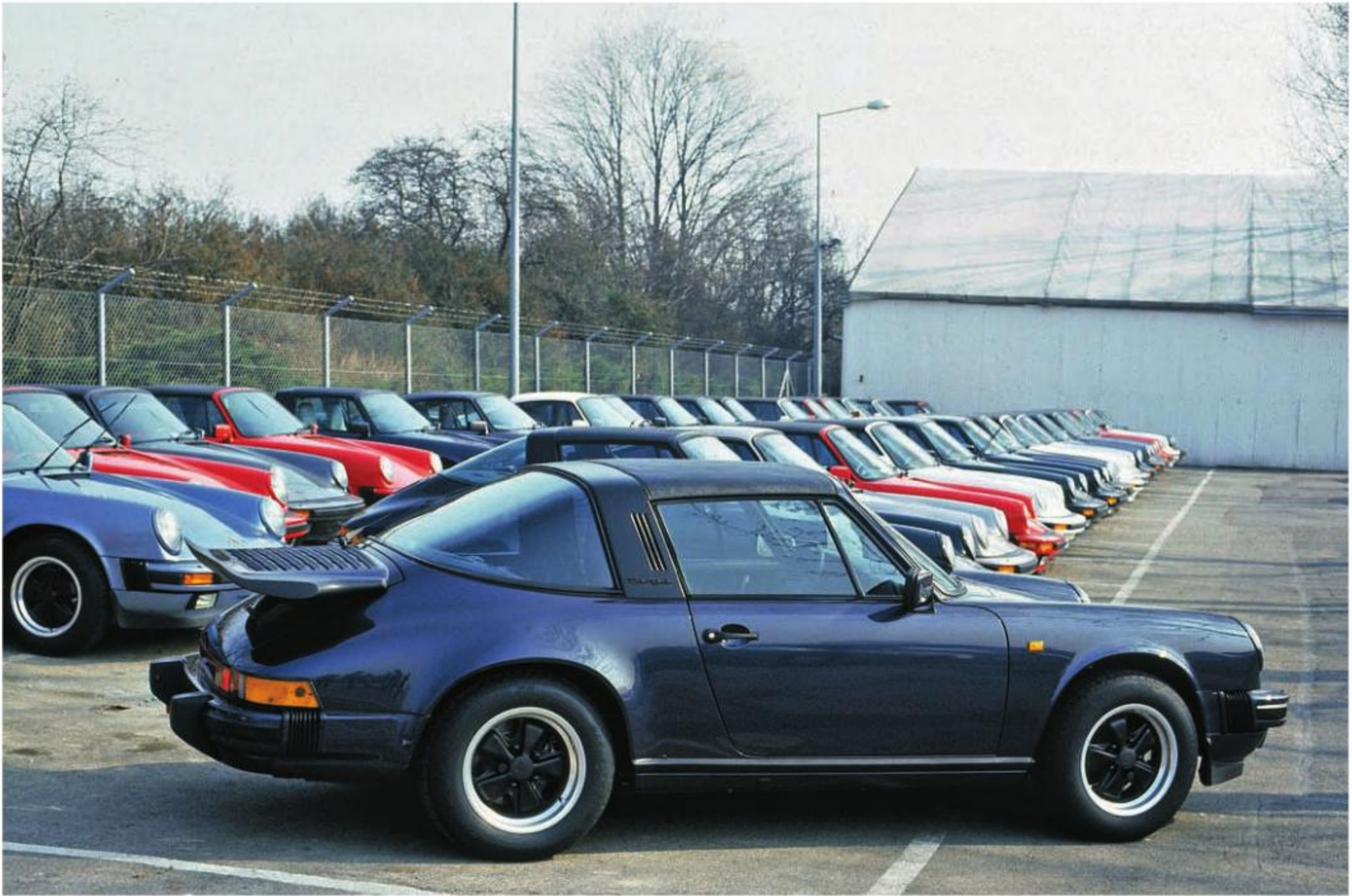
Customers could order new Carrera 3.2 models with flat Turbo-style rear wings and polyurethane front "chin" spoilers as regular production options. Tony Lapine's stylists toned down nearly all the "bright work" to anodized black.
