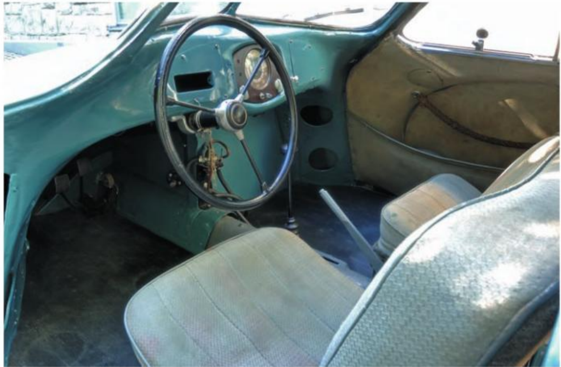
A large-capacity 50-liter fuel tank intruded into the passenger footwell, forcing Porsche to design the car with staggered seating, placing the passenger slightly behind the driver. On a bright day, the interior is airy, but the space is cramped and crude.
