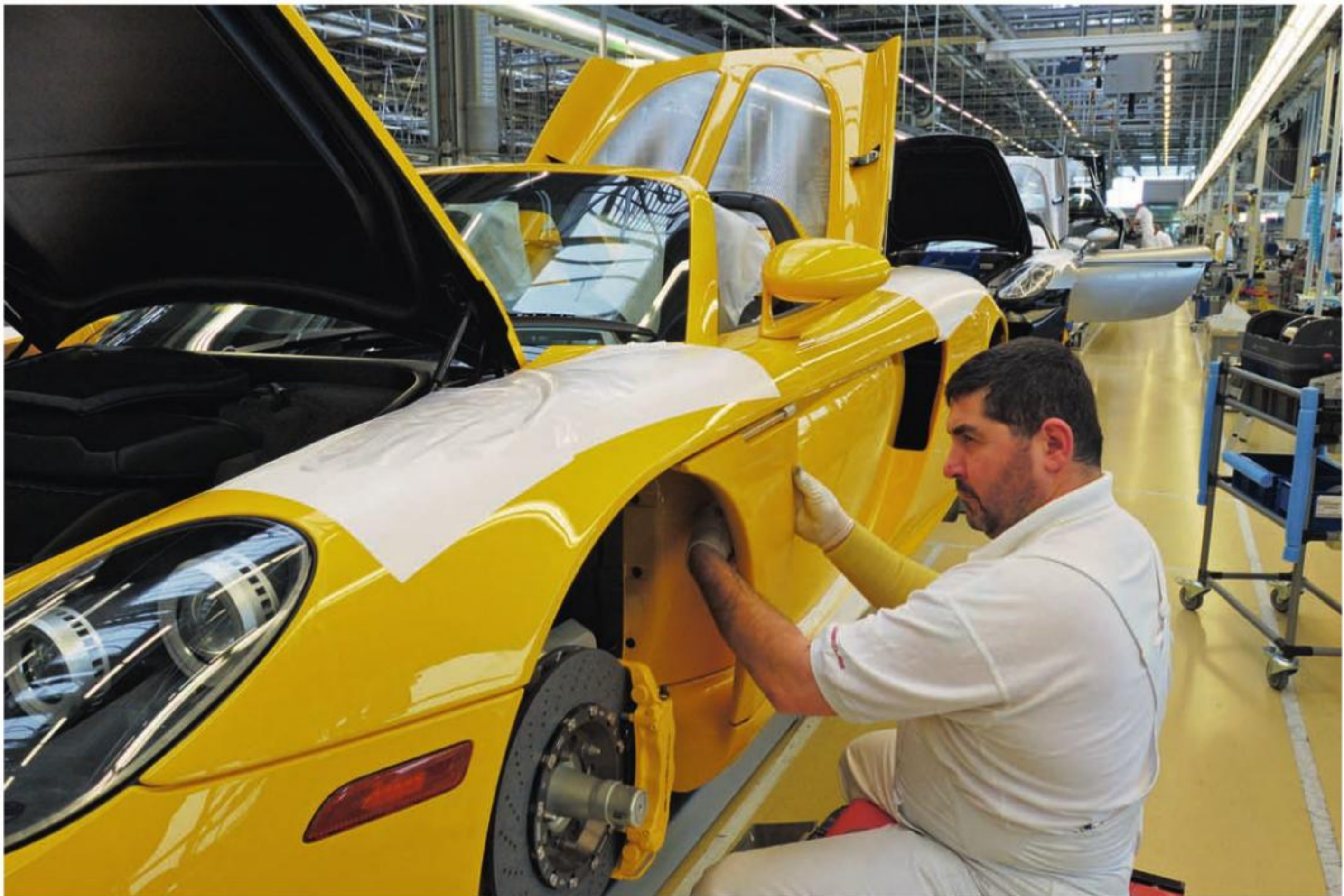
Appearance is everything, especially in a supercar. Here, an assembly technician aligns gaps on front quarter panels, trusting his eye before using a gauge to verify separations.
