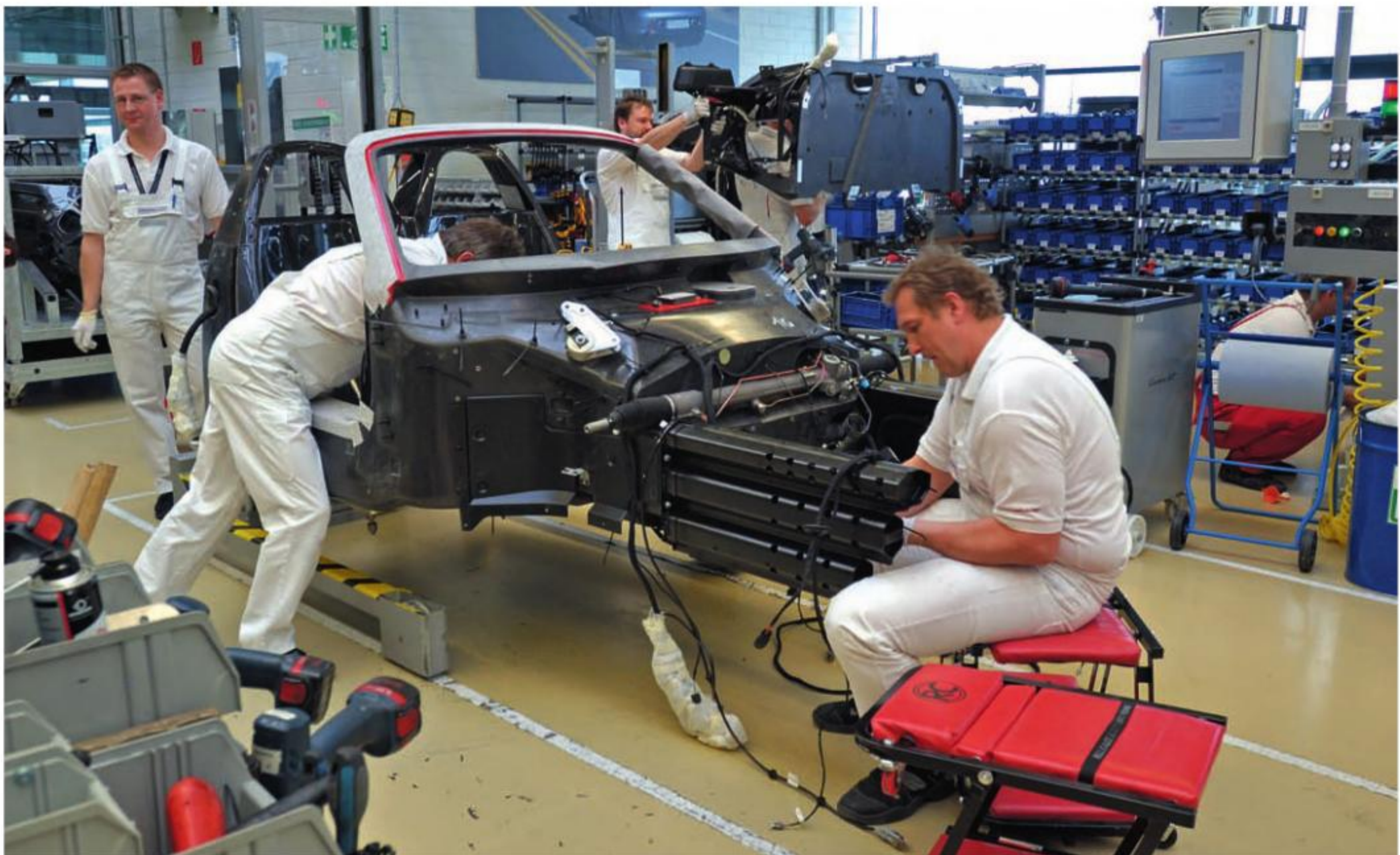
While a team of workers in the background assemble the engine support framework, one waits to attach it to the tub where another technician secures seat mounts. At front a fifth worker threads the wiring harness through the steel compressible structures that make up the car’s crash safety.
