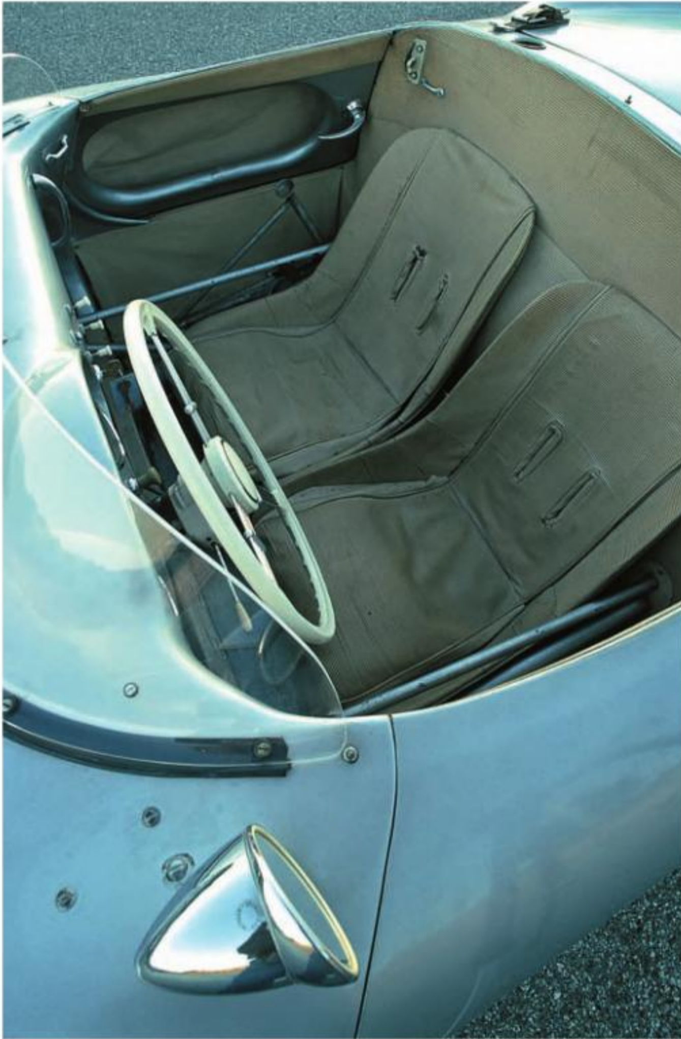
Drivers and occasional co-drivers or navigators had to make do with padded seats in the 550s. The seat back slots were for cooling, not access for lap or shoulder belts.
